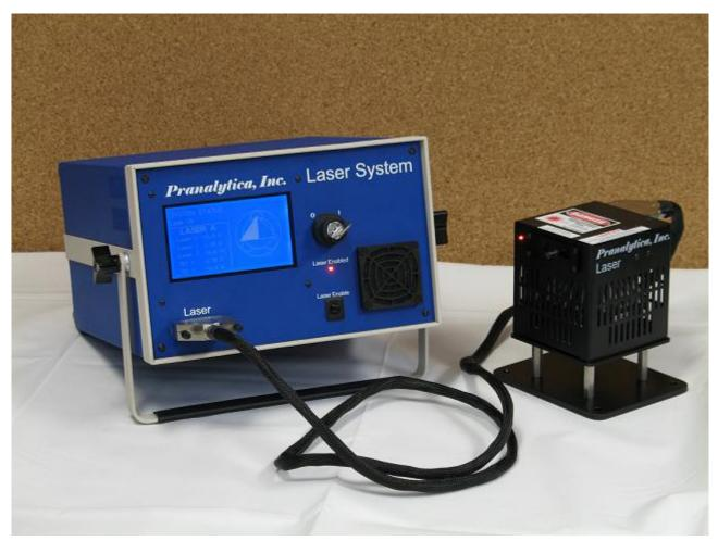
The Model 1101-46-CW-XXXX laser is sold as a complete system consisting of the laser head and matched power supply, ready to be turned on at the customer's location. The thermoelectric cooler and collimating optics for the quantum cascade laser are located in a hermetically sealed package for trouble free operation in real environments.
