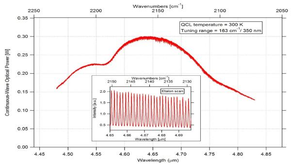
Tuning characteristics of Model 1101-46-EGC quantum cascade laser
